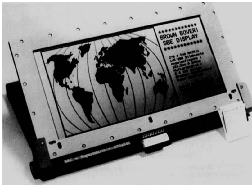
FIGURE 16 Example of image displayed on a super twisted birefringency effect display. (Courtesy of BBC, Brown, Boveri & Co. Ltd.)
